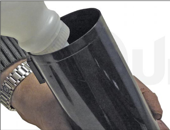
3. Vacuum the tube clean and fill with new replacement toner for use in Phaser 7760.
