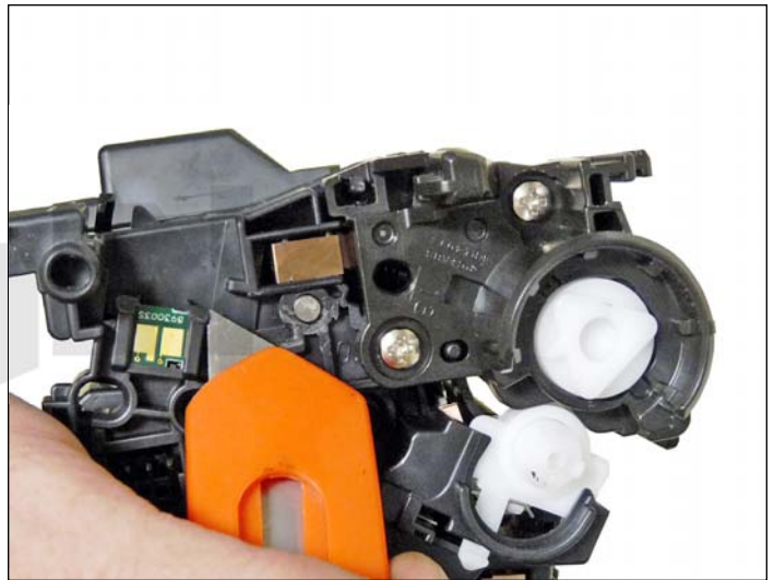
51. Remove the chip by cutting the plastic off the edges of both side of the chip.
