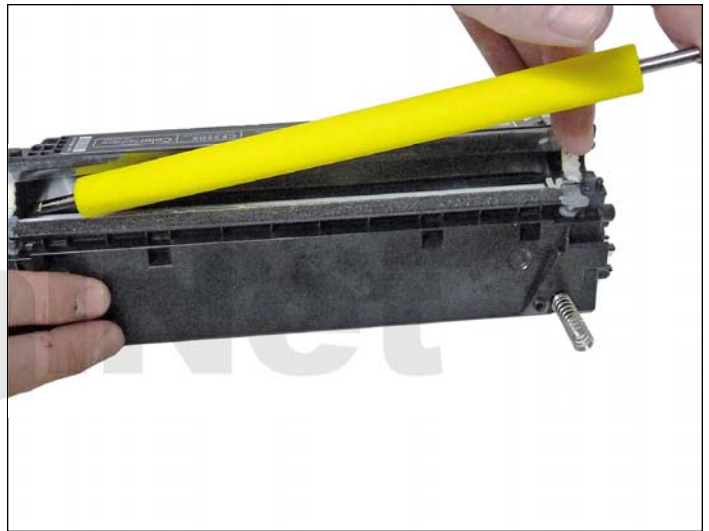
32. Remove the feed roller.
