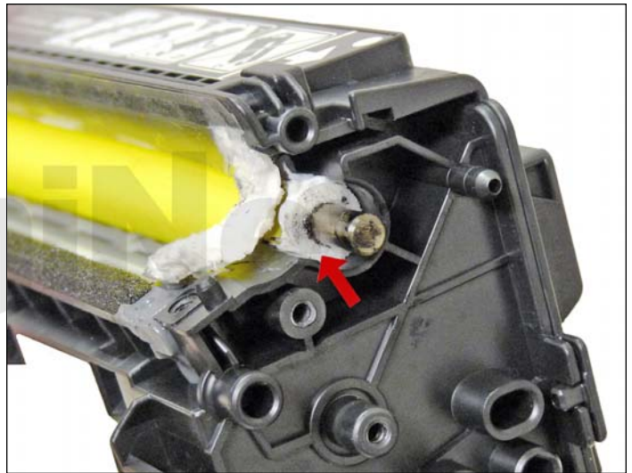
30. Remove the white felt washers from both sides of the developer roller.
