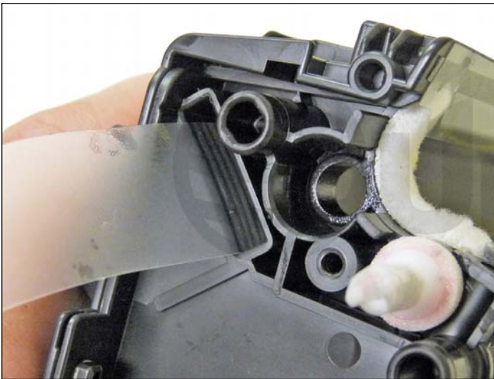
35. Remove the seal port and slide the seal pull tab through the slot.
