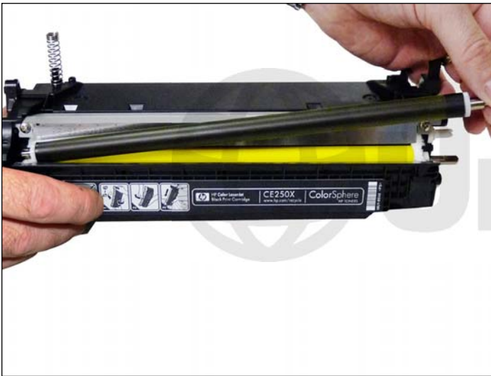
25. Remove the developer roller.
