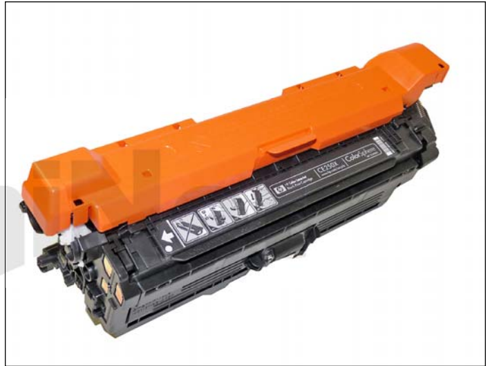
53. Install the drum cover on to the cartridge.
