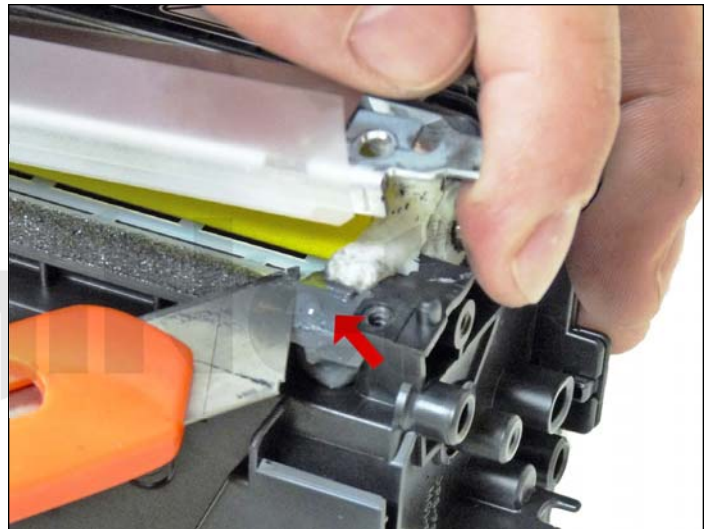
28. Remove the two screws from the doctor blade and start to lift the blade up.
