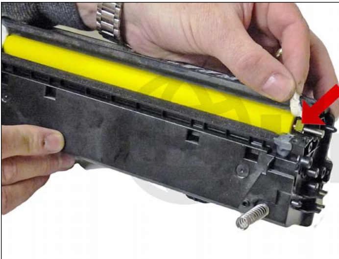
36. Install the feed roller and bushing.
