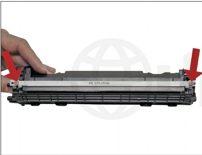
16. Remove the doctor blade and two screws.
