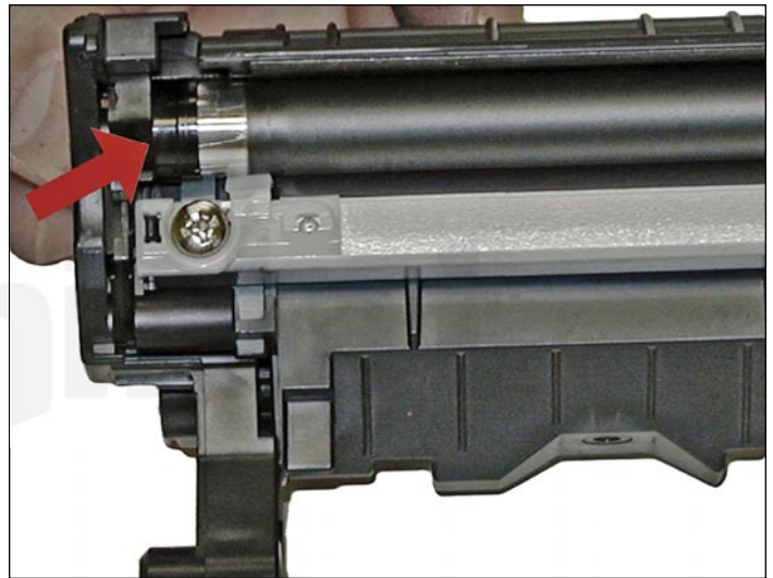
22. Install the magnetic roller black bushing side first.
