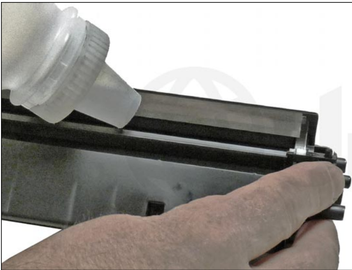
18. Fill the hopper with new toner for use in HP P1102.
