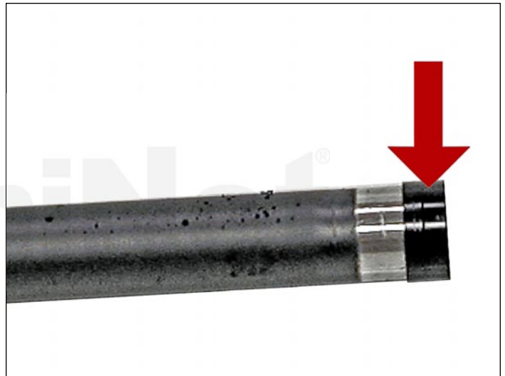
15. Remove the magnetic roller assembly.
