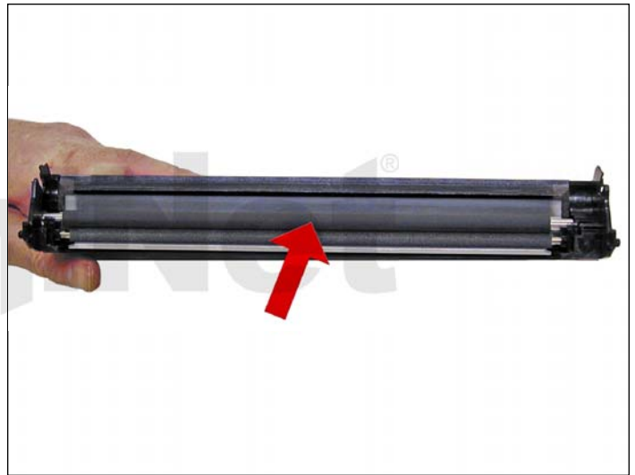
16. Place a small amount of conductive grease in the holders and install the PCR.
