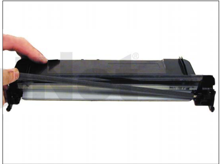
9. Remove the PCR cleaning roller. Clean the PCR with your normal PCR cleaner. WARNING: Do not clean the OEM PCR with alcohol, as this will remove the conductive coating from the roller. If the PCR is an aftermarket, follow the cleaning methods recommended by the manufacturer. If the PCR is an OEM, we recommend it be cleaned with your standard PCR cleaner.
