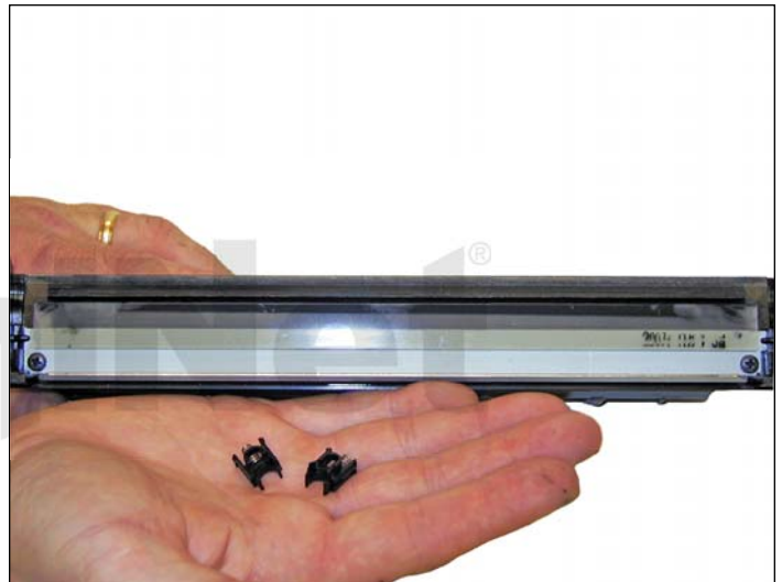
10. Remove both the PCR holders by pressing in on the tabs at the bottom of the holder.
